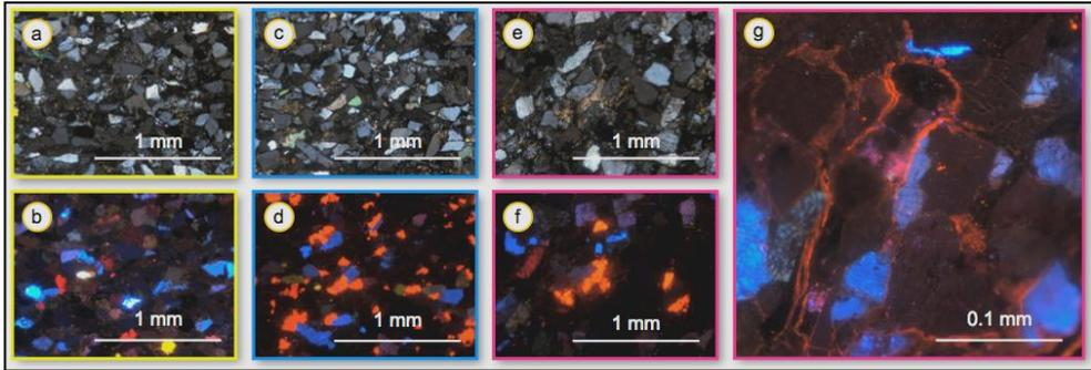
*Fig. 3: a - b) Thin section of the Phnom Bakheng sandstone (PB) and c - d) of the restoration material (PBr). e, f, g) Thin section of the weathering crust. a, c, e) Samples under polarized light and b, d, f, g) under cathodoluminescence. g) Detail of sample under CL showing the finely precipitated calcite within cracks and along the grain boundaries between grains of quartz (very low luminescence) and feldspar (blue). Coloured image frames correspond to the figures below.*
